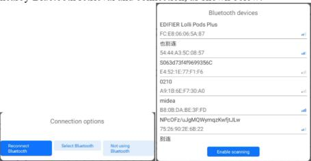
When clicking on 'Reconnect Bluetooth' in the image on the left, it can automatically reconnect to the Bluetooth that has already been connected. Clicking on 'Select Bluetooth' will expand the Bluetooth detection popup on the right. Click on 'Scan and Retrieve Nearby Bluetooth', and then click on the Bluetooth in the list to connect
