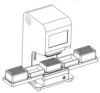
According to the experimental requirements, place the corresponding consumables in the standard SBS plate position. The fit between the consumables and the board position should have no damping sensation, and the flatness of the consumables should not be abnormal. The
