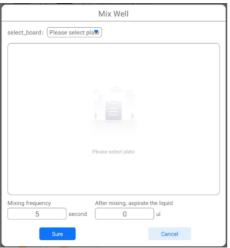
Select the location where the sample needs to be mixed, set the number of mixing times and the amount of liquid absorption after mixing, and click Sure to execute this function.
