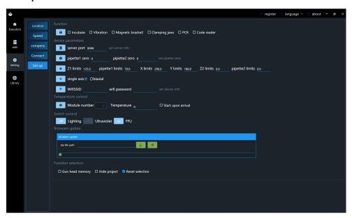
**Module selection:** After checking the box, click the save icon on the left side to use the module and steps when editing the program.
