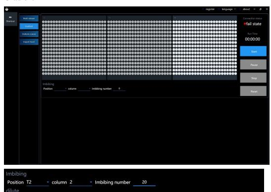
Step 1: Set the imbibing position, set the column and imbibing number after success, and the **dilution** function can be displayed after the setting is completed.
