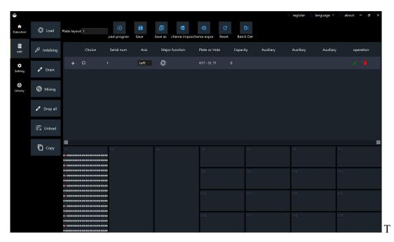
he left button is the main function button, click to edit the corresponding function step, the head button is the scheme related button, the middle part is the scheme list, and the bottom is the position.
