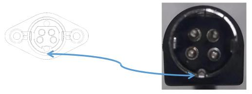
The convex point corresponds to the direction, and then the plug is the correct position
