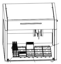
According to the requirements of the experiment, the corresponding consumables are placed in the standard SBS position, and there is no damping sensation between the consumables and the plate level, and the flatness of the consumables is not abnormal, the surrounding gap is moderate, and there is no large shaking sensation, which is normal. (For more information, watch the teaching video)
